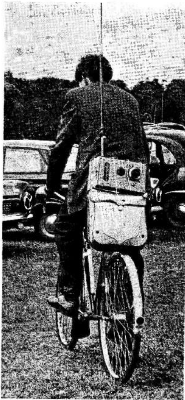
A very keen member of the Bristol A.R.C. is SWL J. Hooper, who turned up at the Longleat Mobile Rally, complete with his /P Rx, having cycled all the way. The gear, which is not actually used mobile for obvious reasons, is entirely home-constructed and enables Jeremy to go out portable-listening on 160 metres. The enthusiasm of our SWL's is surpassed only by their ingenuity.
