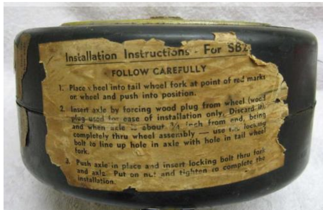
Plan View of SB2C tail wheel with mounting instructions
