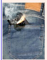
Lithium-ion batteries are used in portable devices because they are lightweight and efficient, but when they short circuit, their liquid components can vaporise and catch fire.
