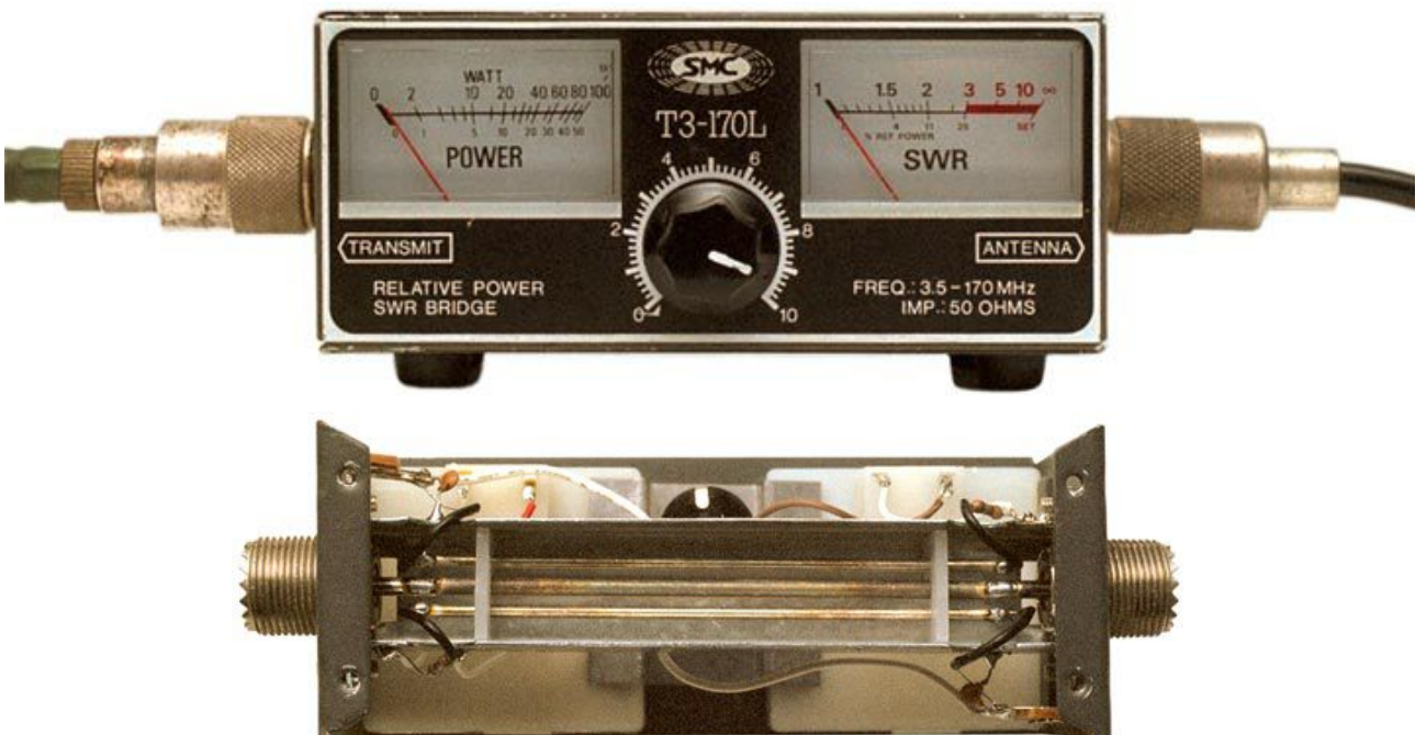
A commercial Sontheimer-Korman reflectometer designed for the Amateur Radio market. (Photographs: D W Knight, www.g3ynh.info/ )
