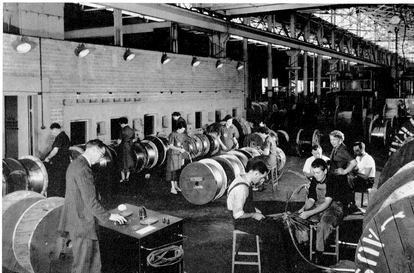
14. On this page are shown the testing of completed cables. Below, test leads are connected to the cable ends and above is the alternating-current test room where cable frequency characteristics are checked.
