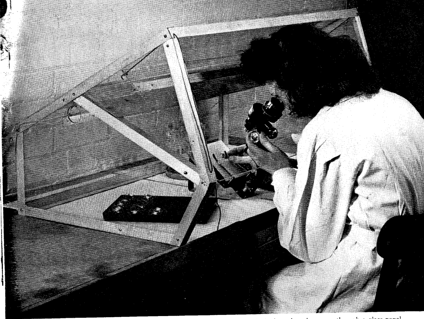
Figure 12—Inspection position for trustworthy valves. The operator looks into the microscope through a glass panel.
