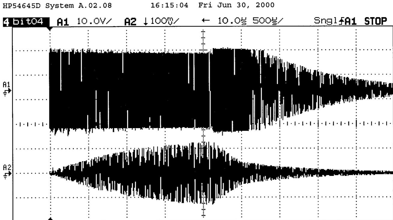
Figure 9: Tesla Coil Voltage and Current Waveforms
