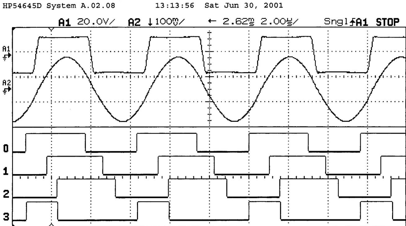
Figure 8: Tesla Coil and Controller Waveforms after 1 ms
