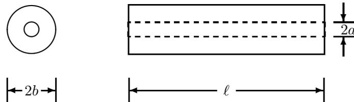
Figure 5: Coaxial Cable
