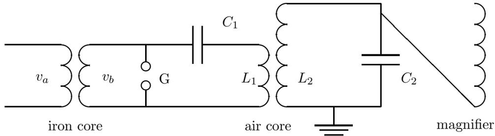
Figure 6: The Classical Tesla Coil With Extra Coil
