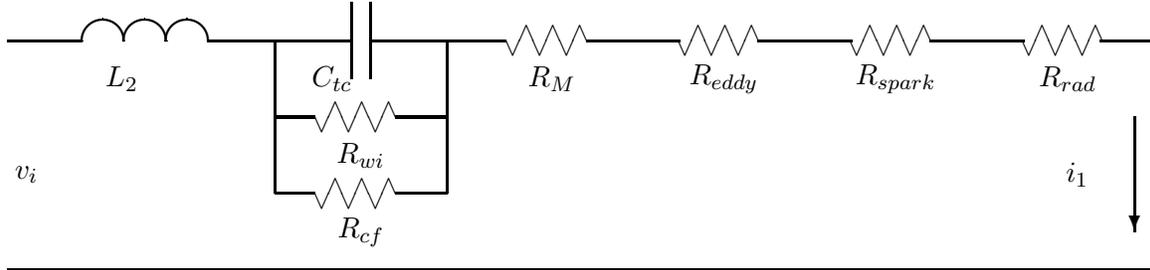
Figure 7: Detailed Lumped Model of Tesla Coil
