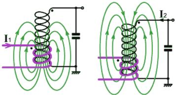
where the field-lines are spreading-out. Hence most of the flux will fail to link with the primary, and the secondary leakage inductance will be large.
