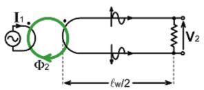
terminals. The two waves combine at the terminals to produce a contribution to the output voltage, because they produce equal and opposite displacements of the terminal potentials.
