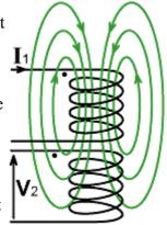
Recall that the self-inductance of a coil is defined as the number of flux linkages per unit current. It follows that, in the case where current in one coil produces flux linkages in another; there is a parameter, having units of inductance, which will allow us to calculate the induced voltage. That parameter, not surprisingly, is called the *mutual inductance*, and is defined as: 'the number of flux linkages in coil 2 per unit of current in coil 1'; i.e.:
