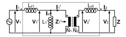
Some comments regarding symbols and notation might be of value at this point. Notice that the leakage inductances are are given the subscript 'x', which should be taken to stand for 'extra'. The high-voltage overwind of a voltage-magnifier transformer is sometimes referred-to as the 'extra coil', and the underlying concept is exactly the same as it is here. Also, using the letter 'l' for leakage has the problem that it is indistinguishable from the figure 'l'.
