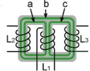
equations, it is possible extract the  $A_L$  values for the magnetic paths a, b, and c (this has already been demonstrated in section 18).
