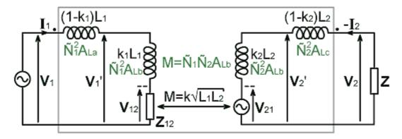
The magnetic coupling can be represented analytically using an ideal transformer having turns  $\tilde{N}_1$  and  $\tilde{N}_2$ . Furthermore, as discussed in the preceding section; the ideal transformer can be represented as a perfect transformer with an inductance  $k_1L_1$  in parallel with its primary port to provide the magnetising current. The redefined network is shown below:
