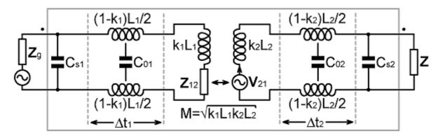
As energy flows through a transformer, each winding causes a delay equal to the time it takes for an electromagnetic wave to travel half the length of the conductor. Velocity is distance divided by time, and so:
