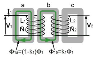
and if we bear in mind that flux  $(\Phi)$  is the counterpart of current; inductance factor  $(A_L)$  is the counterpart of conductance (G); and MMF  $(\tilde{N}I)$  is the counterpart of EMF (V); then it is apparent that we can produce expressions for the partial fluxes  $\Phi_a$  and  $\Phi_b$ .
