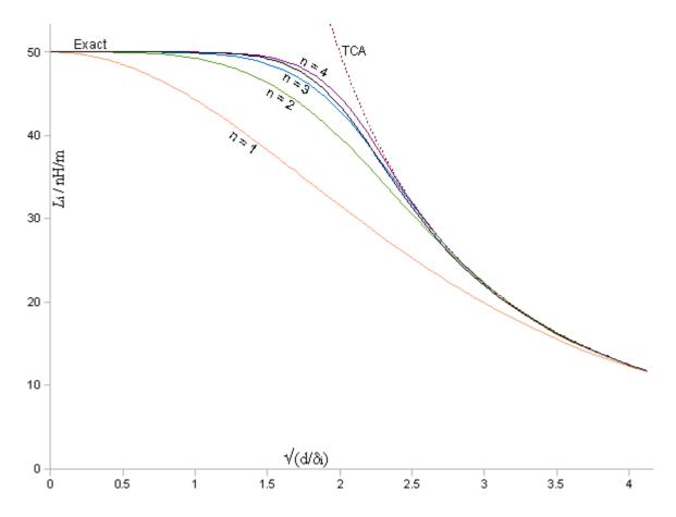
The n=1 case is a rather poor approximation, and best promise is shown for n in the 3 to 4 region. Error curves are plotted below.
