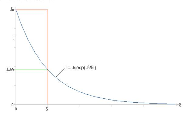
$J_0$  is the magnitude of the current density at the surface of the conductor, and the skin depth  $\delta_i$  is defined such that the area  $J_0\delta_i$  is the same as the area under the decay curve:
