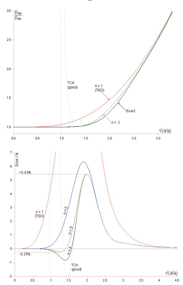
The graphs show that if the ACA is to be used without further correction, the best integer choice for n is 3. Increasing the order beyond 3 has no effect on the maximum positive error, but starts to increase the maximum negative error. Hence, a continuous formula for  $A_{\text{eff}}$  accurate to within 5.5% is:
