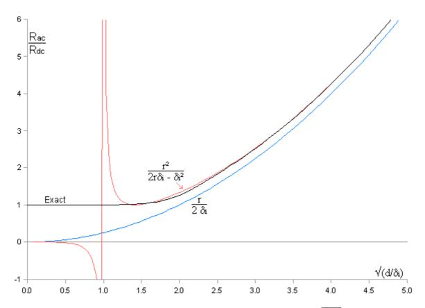
The 'good' approximation goes to infinity when  $d=2r=\delta_i$ , i.e., when  $\sqrt{d/\delta_i}=1$ ; but then converges rapidly with the exact calculation as  $d/\delta_i$  increases. If the formula is used for  $\sqrt{d/\delta_i}>\sqrt{2}$ , i.e.,  $r>\delta_i$ , the maximum error is 5.5%. As a practical example; for a 0.5 mm diameter copper wire,  $r=\delta_i$  at 700 kHz.
