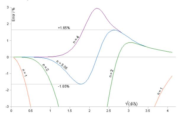
Values of n in the region of 3 produce S-shaped error curves, and n=3.05 makes the positive and negative maximum error magnitudes the same. Hence a simple continuous formula for internal inductance accurate to  $\pm 1.65\%$  is:
