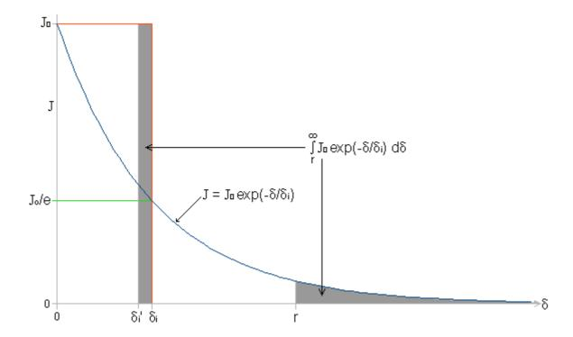
It is not obvious that the truncation should occur at depth r (the wire axis), but proof will be given shortly. For now, observe that the area  $J_0 \, \delta_i$ ' must be the same as the area under the decay curve from 0 to r . Thus:
