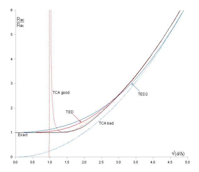
The goodness of an approximation is demonstrated by plotting the difference between it and the exact value, as in the graph below. The curves shown are all calculated from the expression:
