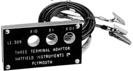
This special adaptor enables in-situ measurements to be made at frequencies up to about 1 MHz.
