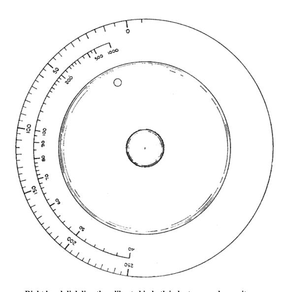
Right hand dial directly calibrated in both inductance and capacitance.
