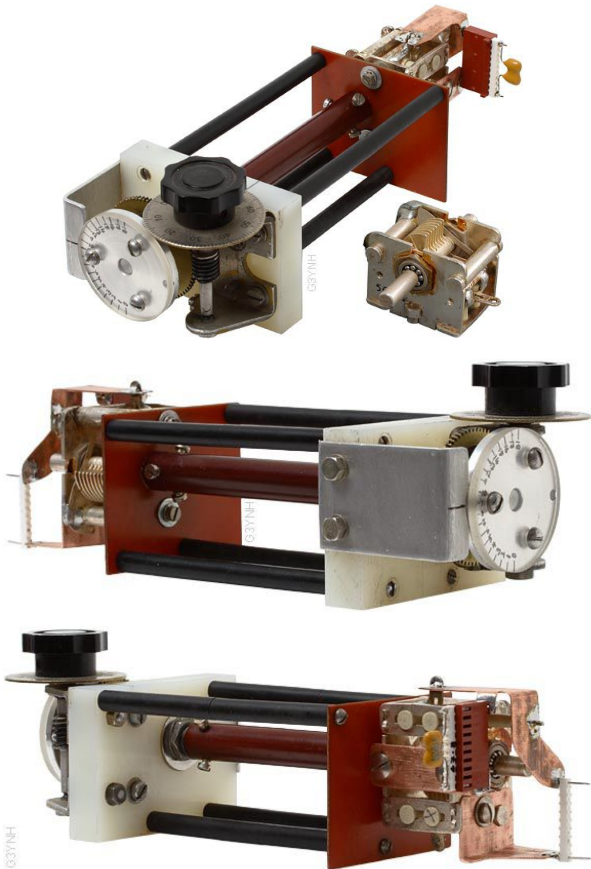
40 pF variable reference capacitor with 36:1 anti-backlash worm drive ( capcal_8-48.ods ). A socket is provided for a parallel padding capacitor
