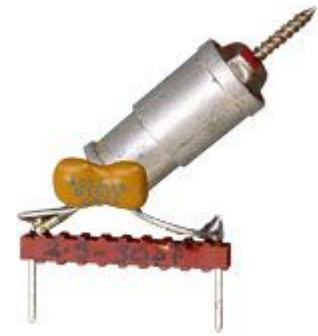
Silver-mica capacitor and 2.5 pF - 30 pF trimmer
