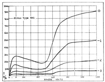
The valve was tested in a normal 3-valve battery receiver and the gain was found to be  $+12\mathrm{db}$ , actually higher than a normal screened grid, presumably due to the incidental reaction caused by the higher inter-electrode capacity. The valve was found to be entirely non-microphonic.
