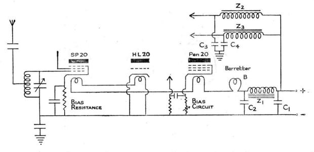
mains supply and must be connected in series, the voltage drop across each heater being approximately 20 volts. It is essential that the heater current be maintained absolutely constant at 18A. The most satisfactory method of
