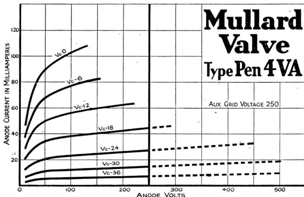
Owing to its high effective amplification it may be used in all A.C. mains receivers having no other low frequency stage.
