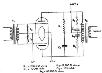
The optimum plate-to-plate load for the P.M.2B is 14,000 ohms, and the resistance of the primary winding of the output transformer, T2, should not exceed 1,000 ohms.
