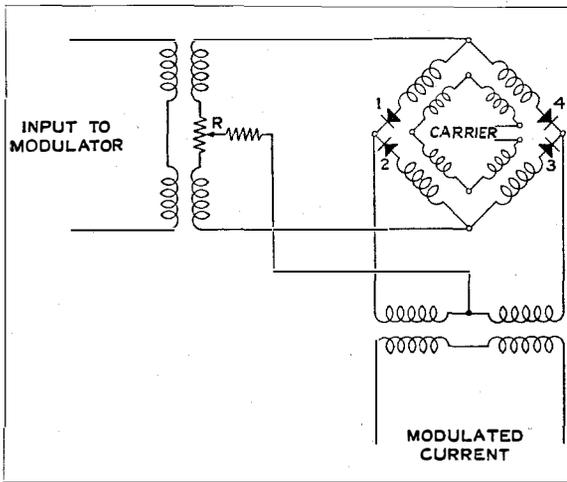
Fig. 3—Modulator Schematic.
