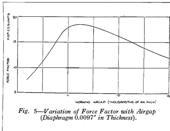
Fig. 5—Variation of Force Factor with Airgap (Diaphragm 0.0097" in Thickness).
