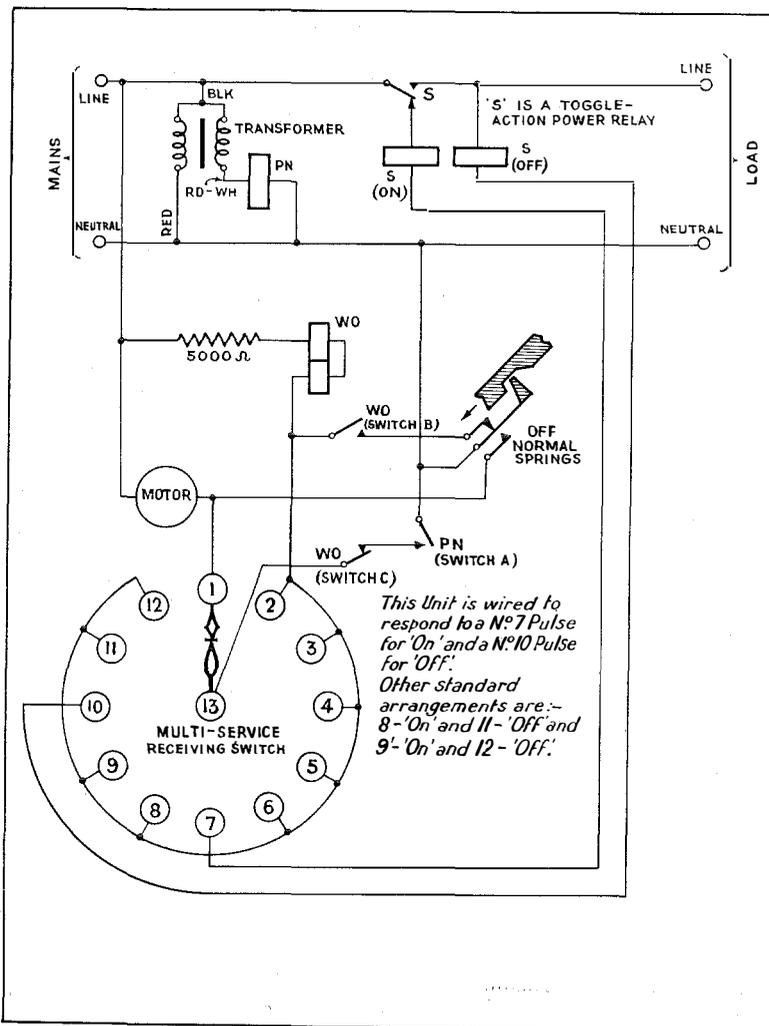
Fig. 9—Schematic Circuit of Multi-service Control Receiving Unit.
