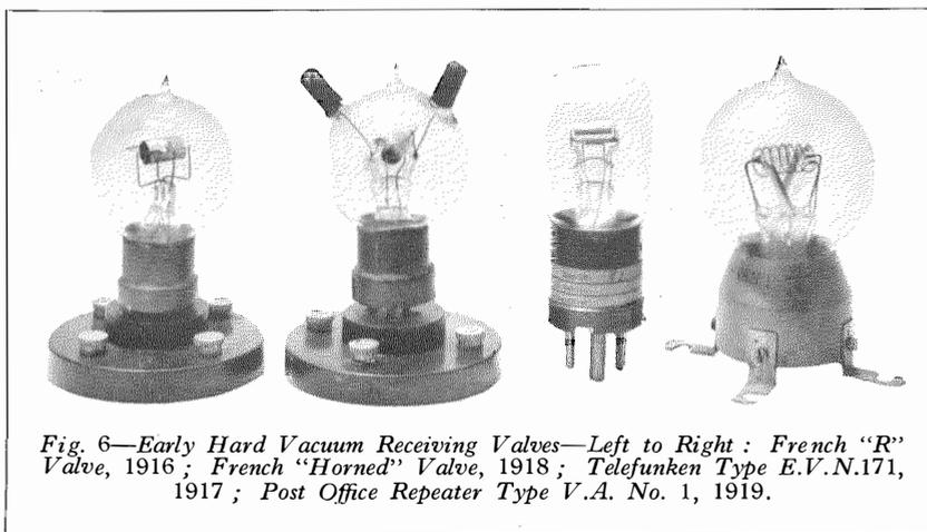
Fig. 6—Early Hard Vacuum Receiving Valves—Left to Right : French "R" Valve, 1916 ; French "Horned" Valve, 1918 ; Telefunken Type E.V.N.171, 1917 ; Post Office Repeater Type V.A. No. 1, 1919.
