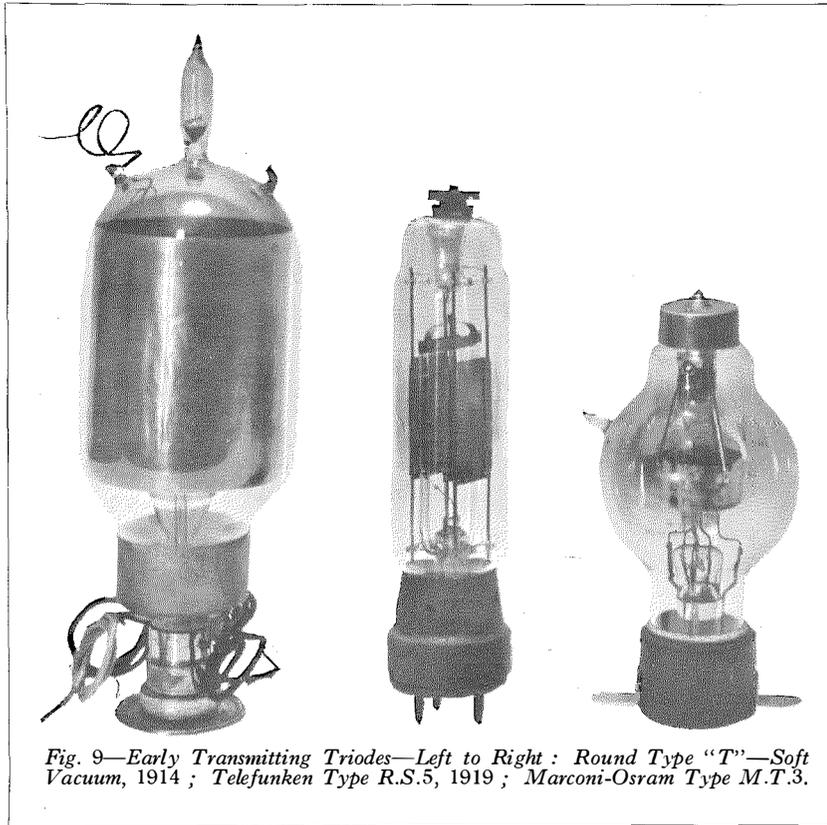
Fig. 9—Early Transmitting Triodes—Left to Right : Round Type "T"—Soft Vacuum, 1914 ; Telefunken Type R.S.5, 1919 ; Marconi-Osram Type M.T.3.
