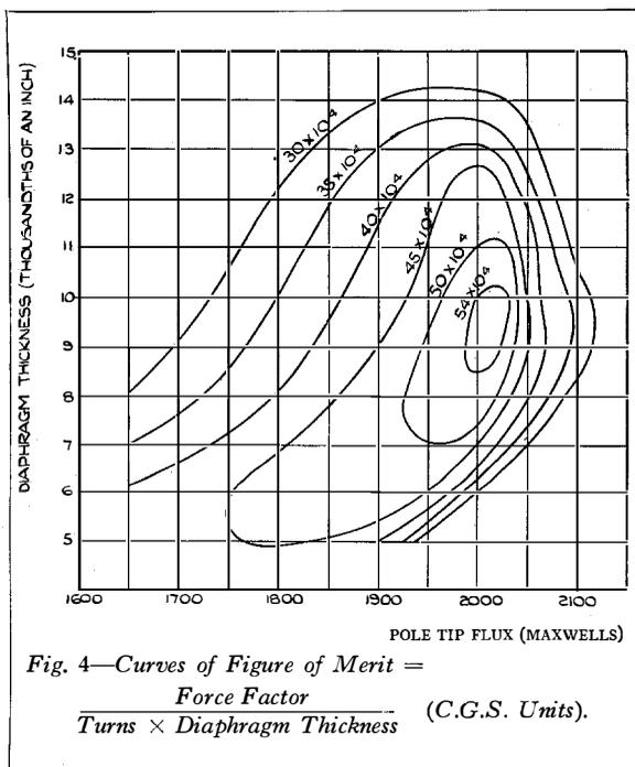
Fig. 4—Curves of Figure of Merit =  $\frac{\text{Force Factor}}{\text{Turns} \times \text{Diaphragm Thickness}}$  (C.G.S. Units).
