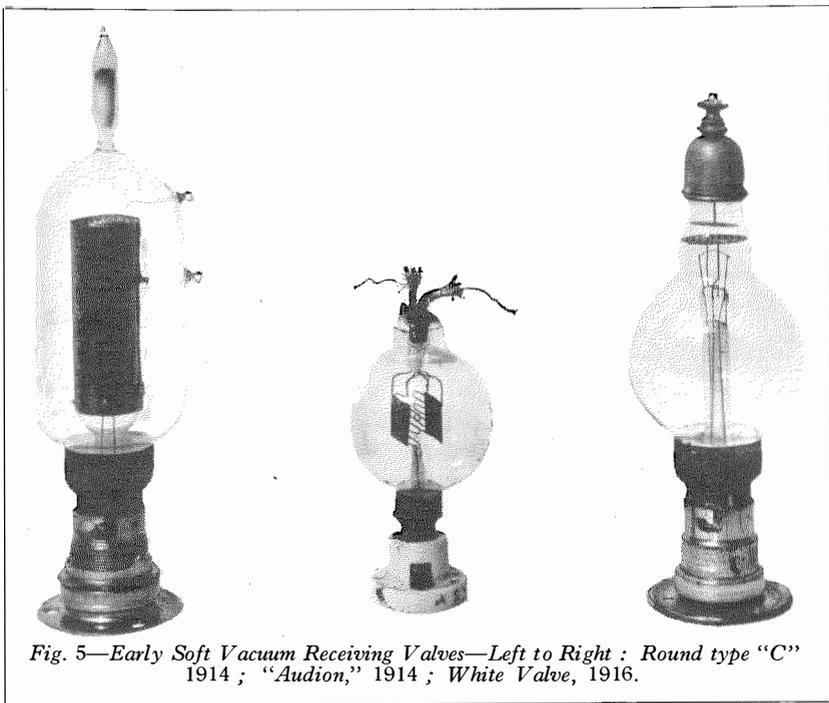
Fig. 5—Early Soft Vacuum Receiving Valves—Left to Right : Round type "C" 1914 ; "Audion," 1914 ; White Valve, 1916.
