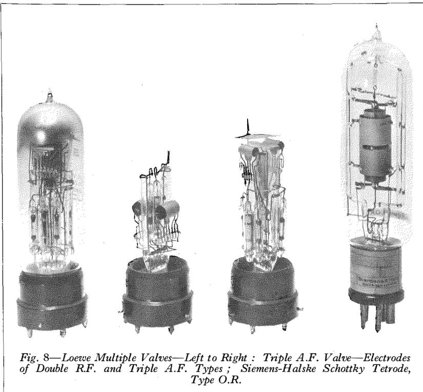
Fig. 8—Loewe Multiple Valves—Left to Right : Triple A.F. Valve—Electrodes of Double R.F. and Triple A.F. Types ; Siemens-Halske Schottky Tetrode, Type O.R.
