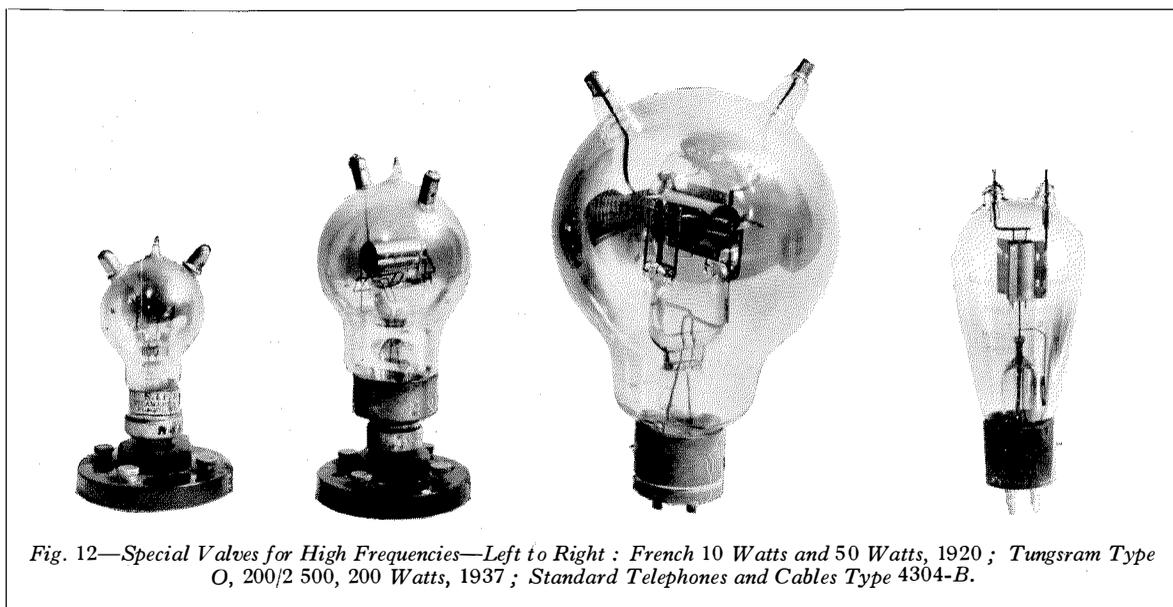
Fig. 12—Special Valves for High Frequencies—Left to Right : French 10 Watts and 50 Watts, 1920 ; Tungsram Type O, 200/2 500, 200 Watts, 1937 ; Standard Telephones and Cables Type 4304-B.
