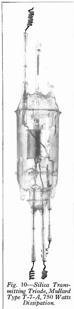
Fig. 10—Silica Transmitting Triode, Mullard Type T-7-A, 750 Watts Dissipation.
