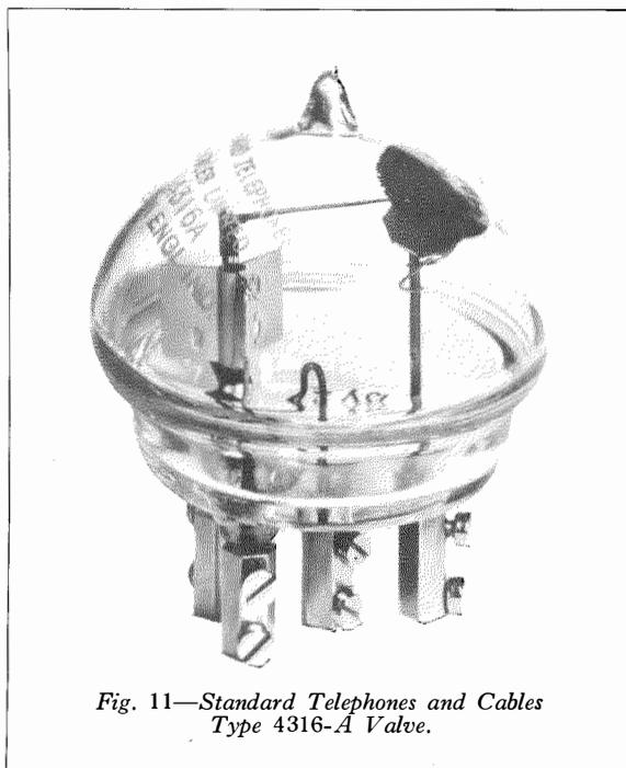
Fig. 11—Standard Telephones and Cables Type 4316-A Valve.
