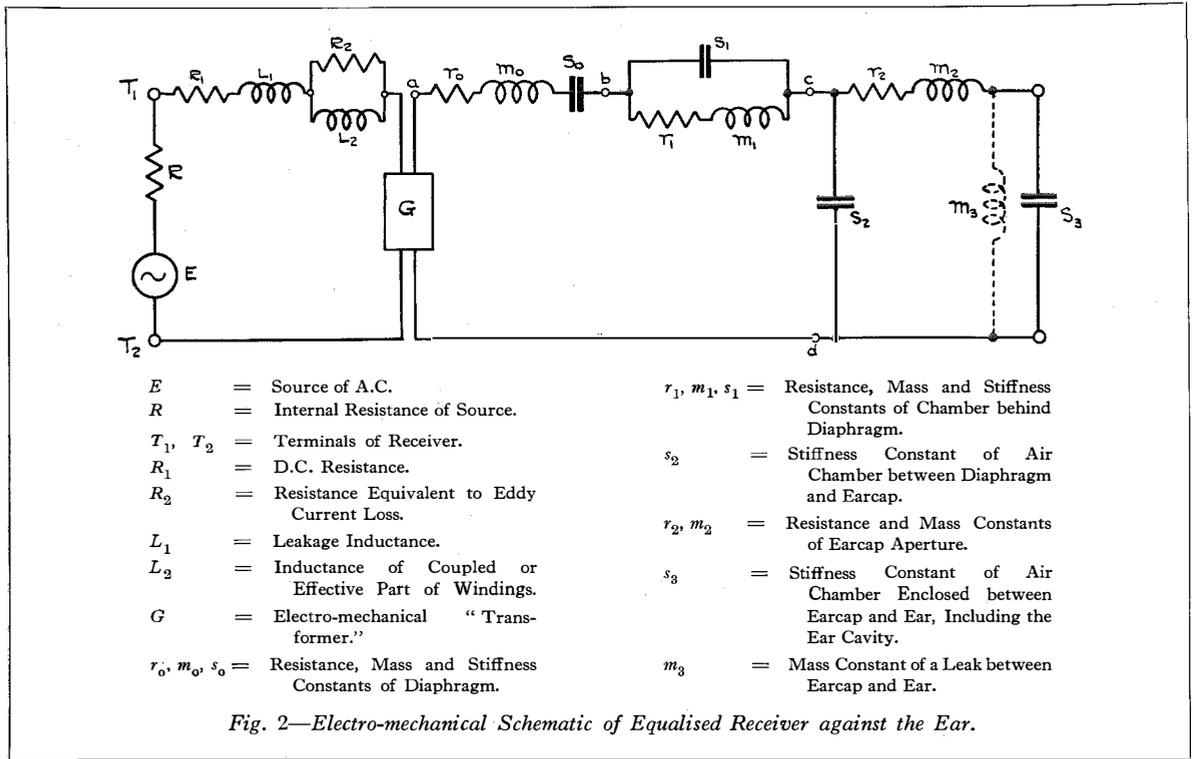
An advantage of the new receiver, due to its damped characteristic, is that the effect on the ear of surges or any abrupt interfering noises in the listener's circuit is much reduced. The energy of a surge tends to set the diaphragm in motion and, when the latter is freely resonant as in the old receiver, the motion persists for several cycles; in a well damped diaphragm system, however, the surge energy is dissipated too rapidly to be fully appreciated by the ear.
