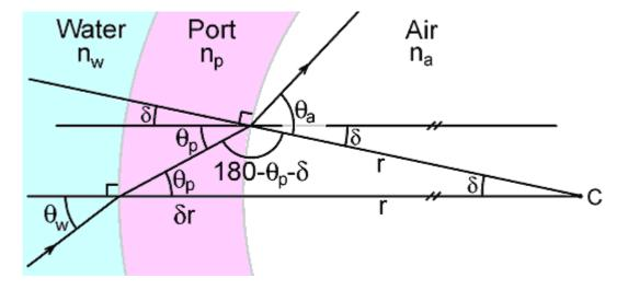
In the diagram above, an incident ray (in water) meets the port surface at an angle  $\theta_w$  to the perpendicular and emerges into the port material at an angle  $\theta_p$ . The relationship between the two angles is given by Snell's law in the small-angle limit:
